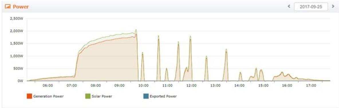
**Figure 14: Screenshot of the overvoltage drop-out on 25 Sep 2017**
