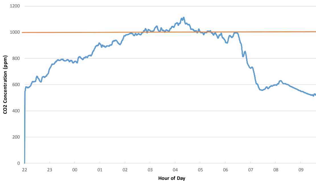
Figure 11: A datalog of one night's CO 2 monitoring in our main bedroom
