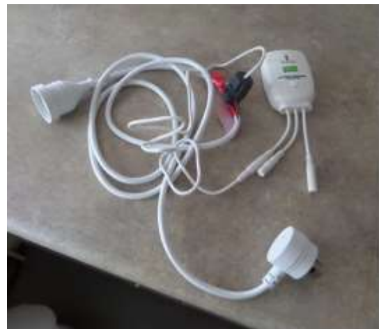
Figure 10: One of the 'cable split' extension cords I have been using for socket level datalogging
